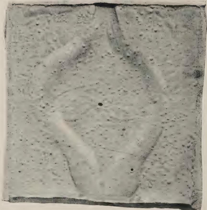
» When the process first began, numerous comparatively small holes would form one after other. These holes would continue to enlarge, retaining their circular form, as the hot liquid was forced through them, until the action was stopped by a sufficiently thick crust forming upon the liquid surfaces. »
